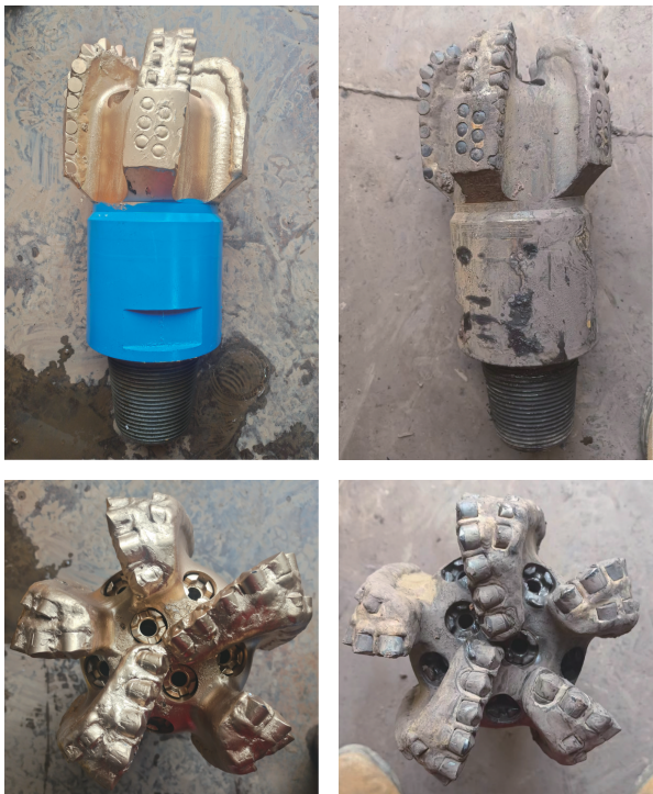
图6 OGS屋脊齿PDC全面钻头入井前后对比 Fig.6 Comparison before and after use of OGS PDC Ax-shaped cutter bit
