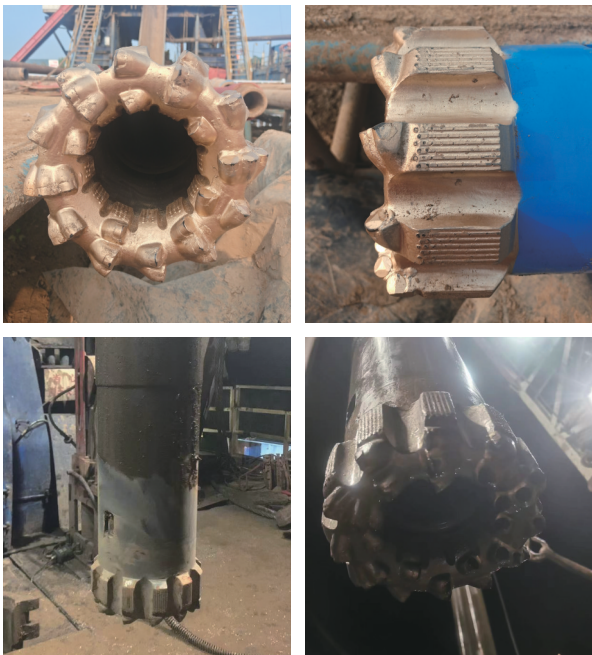
图8 新型平顶三棱齿PDC取心钻头入井前后对比 Fig.8 Comparison before and after use of triangular PDC coring bit
