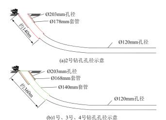
图 5 钻孔结构示意 Fig.5 Schematic of drilling structure
