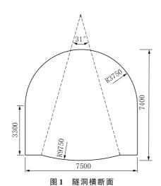
Fig.1 Cross-section of the tunnel
