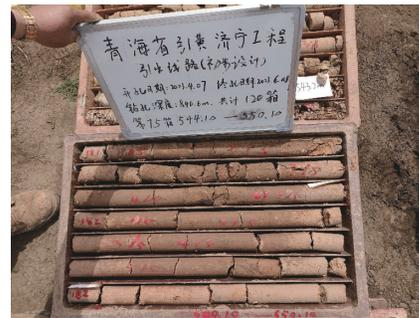
(b)隧洞桩号38+100处SCZK06钻孔(553~560m岩心)
