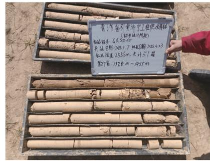
(a)隧洞桩号71+900处SCZK14钻孔(144~150m岩心)
