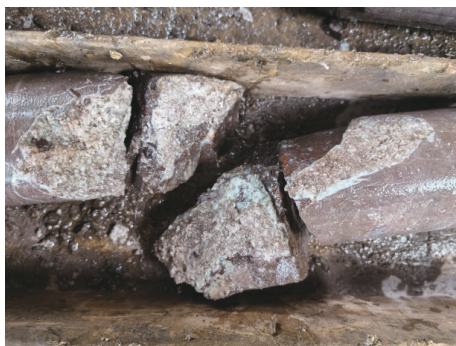
图5 ZK2001裂隙发育段岩心 Fig.5 Core from the fracture development section of ZK2001
