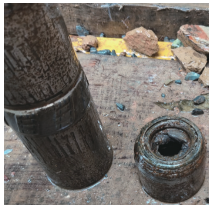
图6 孔底失返非正常损耗的钻头 Fig.6 Abnormal wear bits due to loss circulation at the bottom hole
