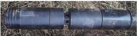
图 11 伸缩式漏液接头 Fig.11 Telescopic leakage joint
