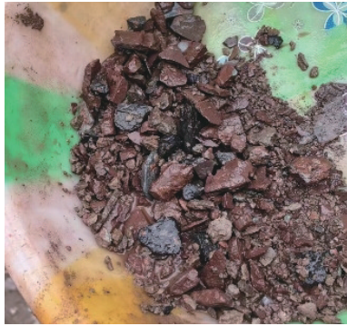
图4 井深2765.00 m处振动筛返出的掉块 Fig.4 The blocks of vibrating screen returned from 2765.00m depth
