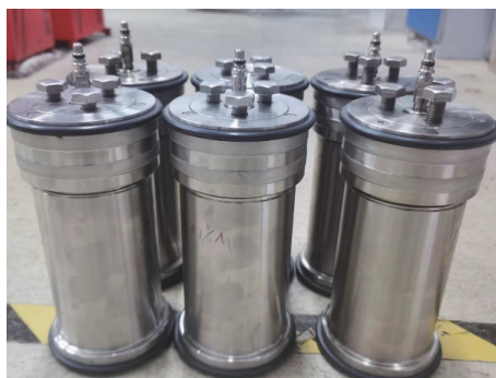
(b) 承压老化罐
