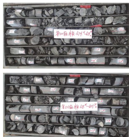
图8 破碎井段岩心 Fig.8 Core of fractured well section
