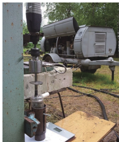
图6 空气洗井钻进实验室试验台外观照片 Fig.6 Exterior Photo of drilling testbed in laboratory with flushing by compressed air
